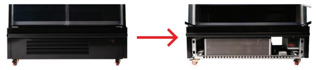
Remove front panel to access condenser. Ensure condenser is cleaned every 6 weeks.
