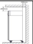
5- To avoid vibrations, the unit must be level.
